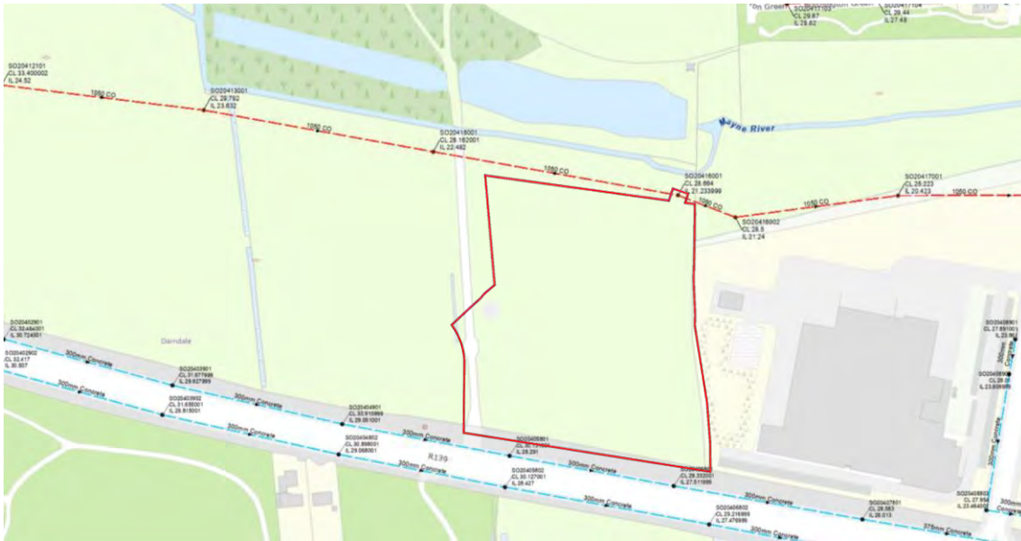
Figure 3-2: Existing water infrastructure
